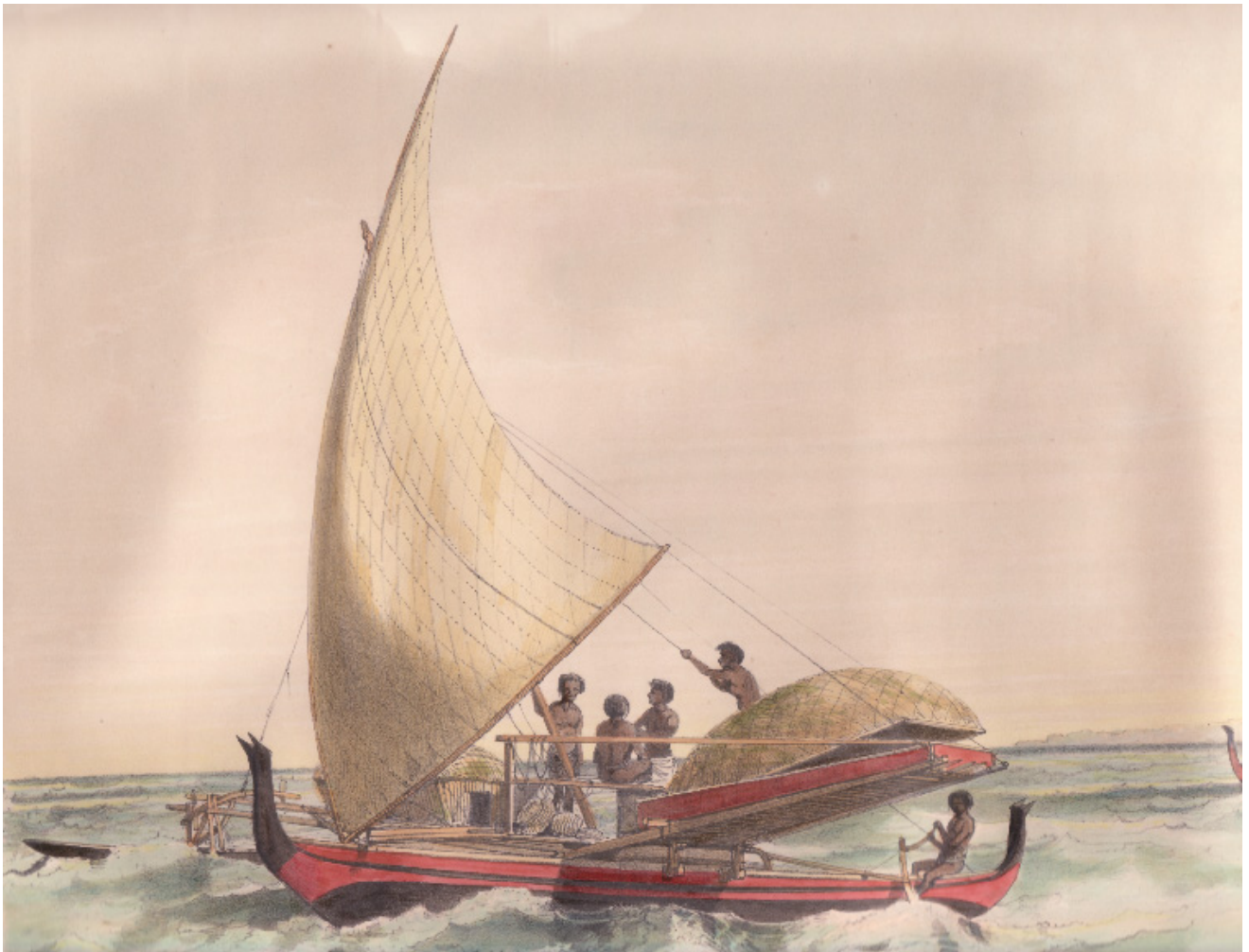
Figure. 5. A single-outrigger travelling canoe of Satawal, in the Caroline Is., Micronesia. This boat was encountered by the French corvette, the Astrolabe , in 1826 and the print was published by Pâris in 1843 (plate 107). The outrigger is on the far side, beneath a little hut with a square door. The sail is held up by a stay to the wide beam on the lea side, which also supports a plaited shelter.
