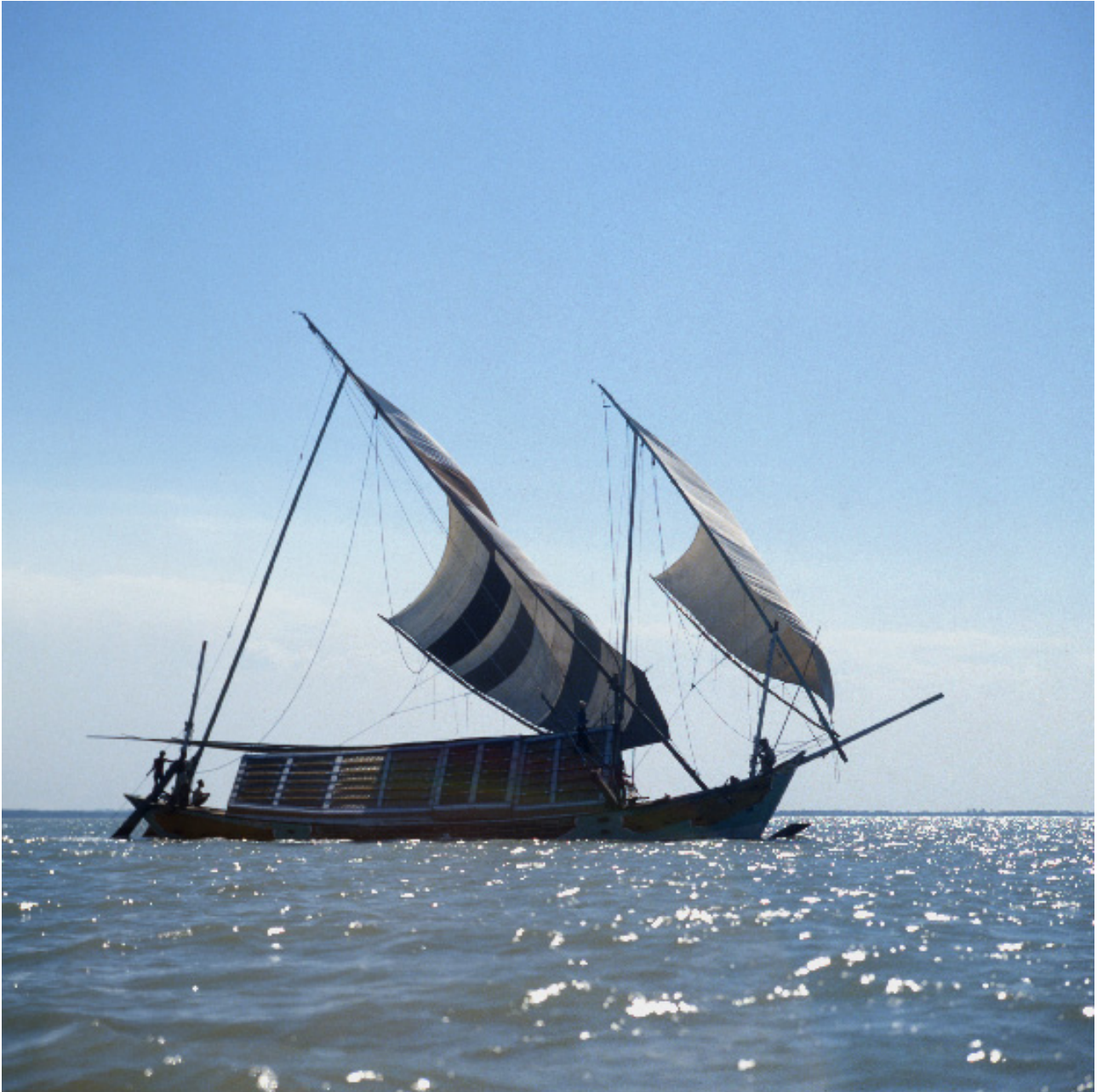
Figure 12. The mastless rig today. This is a Madurese Janggolan sailing downwind heavily loaded with salt. The main is a two-boom triangular sail supported by a pole to the stern and stays to the beams on each side. The fore sail is similar with a sliding ring on the bowsprit. The vertical pole in the stern is a support for the lowered rig. Note the two huge rudders that act as a keel.
