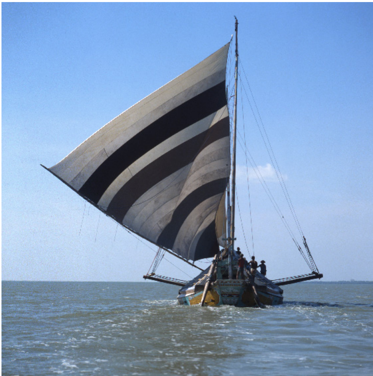
Figure 13. Stern view of the janggolan in figure 12. Note the four stays to the beam on each side, and the way that the shape of the belly of the sail is controlled by the lacing.
